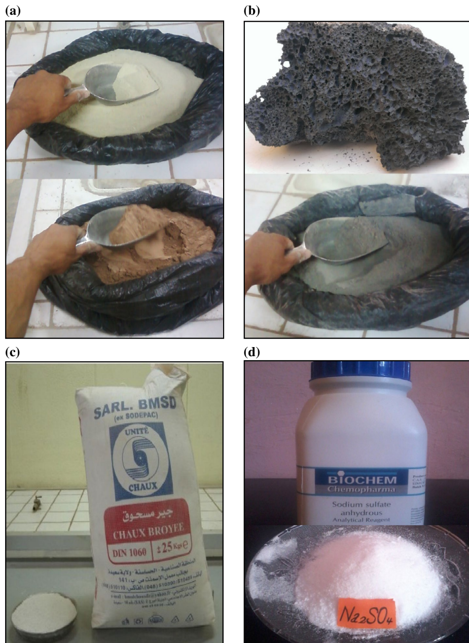
1 Materials used and their preparation a RS sieved to 1-mm sieve, b NP rock ground in the laboratory in order to obtain a fine powder with specific surface area of 420 \text{ m}^2/\text{kg} , c lime typically used for construction purposes and d \text{Na}_2\text{SO}_4
